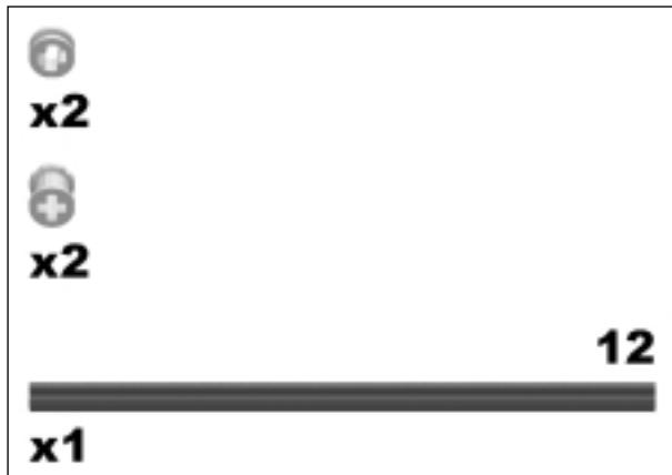
Pass a #12 axle through the beams and the liftarms. Secure it with two bushings on the outside.
