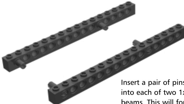
Insert a pair of pins with friction into each of two 1x16 TECHNIC beams. This will form the side frames of the robot base.
