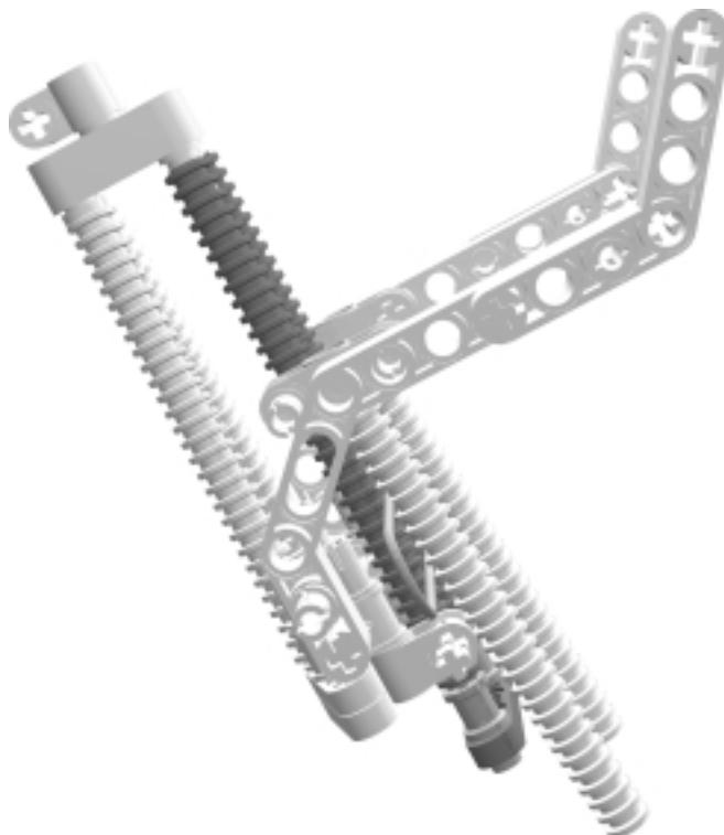
Insert the parts as shown, leaving the yellow elastic band for last. The elastic goes between the green and purple flex hoses and wraps around the black friction pegs (below) that are inserted in the yellow double-bent liftarm. Its purpose is to hold the purple hoses against the front of the loader mechanism. This is important, so study the image carefully.
