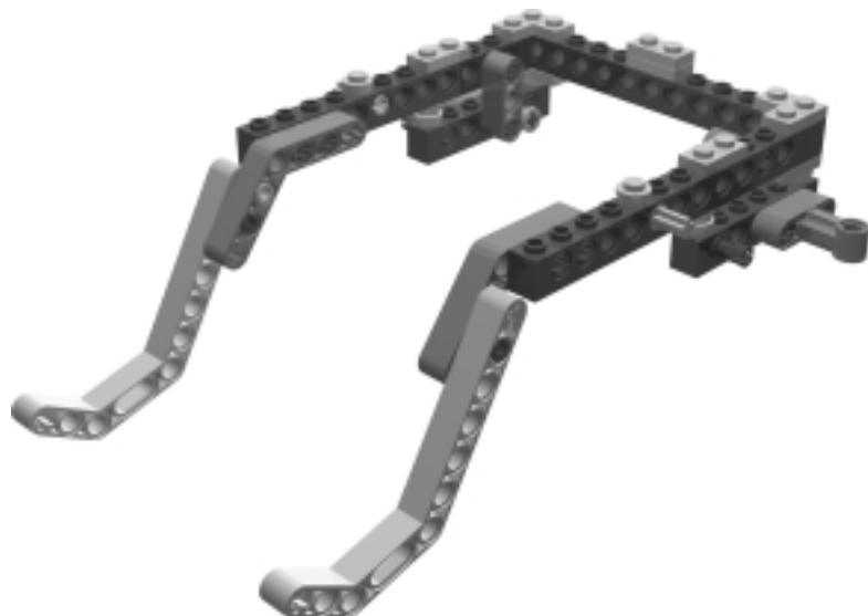
Hopper's chassis is a simple frame onto which all of the other parts are added.
