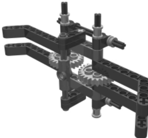
Now you begin the interesting part of HunterBot: the grabber arms. The business end of the grabber “claw” is a simple assembly of four angled liftarms on a series of axles. When the 24t gears rotate, the grabber arms open or close.
