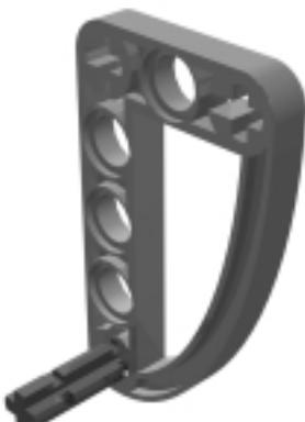
This part of the loader is responsible for pushing each domino out. Insert the #2 axle into the bottom of the blue quarter-oval TECHNIC liftarm. The liftarm is connected to the #3 axle that in turn is connected to the 40t gear. Make sure that the liftarm rotates freely.
