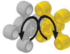
Diagram 2: TECHNIC knob wheel 90 degree coupling
