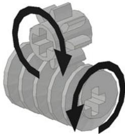
Diagram 3: TECHNIC worm gear. The turning motion must be applied to the screw. Trying to turn the gear will not provide any motion.
