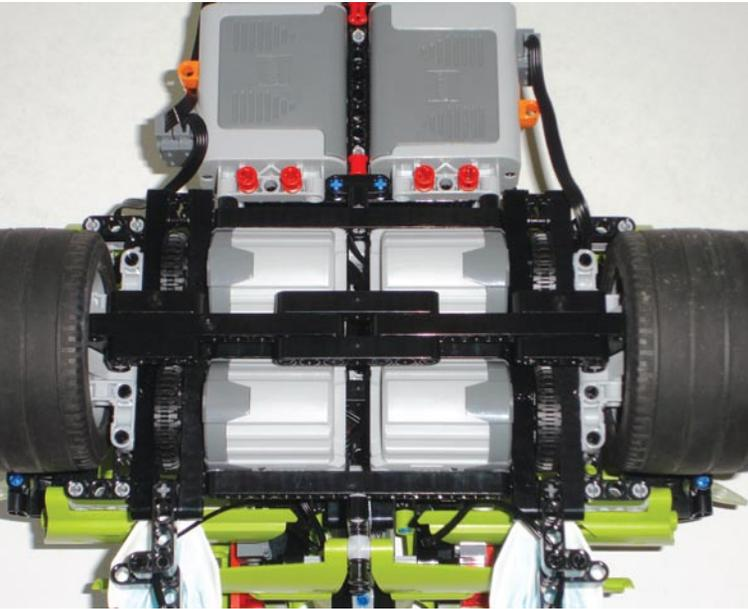
Greenie is propelled by 4 motors from the rear axle. These are XL Power Function motors, which are the larger of the two available Power Function motors. The motors are easy to integrate into a design due to the Technic holes that are in a cross-type formation around the output axle. The 4 XL Power Function motors also provide plenty of power for their size and weight, which make them ideal candidates to be used as part of the drive train.
