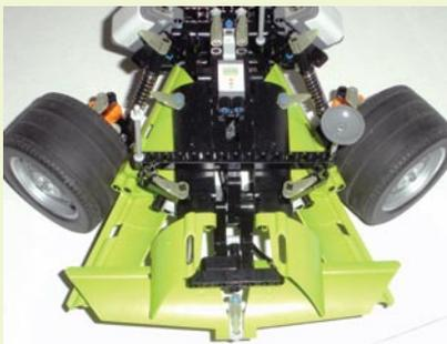
Front steering assembly in emergency stop (top view)
