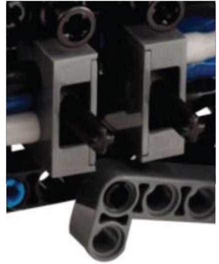
Figure 1: The pneumatic switches.
