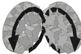
Diagram 4: TECHNIC bevel gear. This acts just like the knob wheel gearing in diagram 2, but the elements are more indicative of real world beveled gearing..
