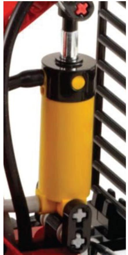
Figure 2: The pneumatic cylinder.
