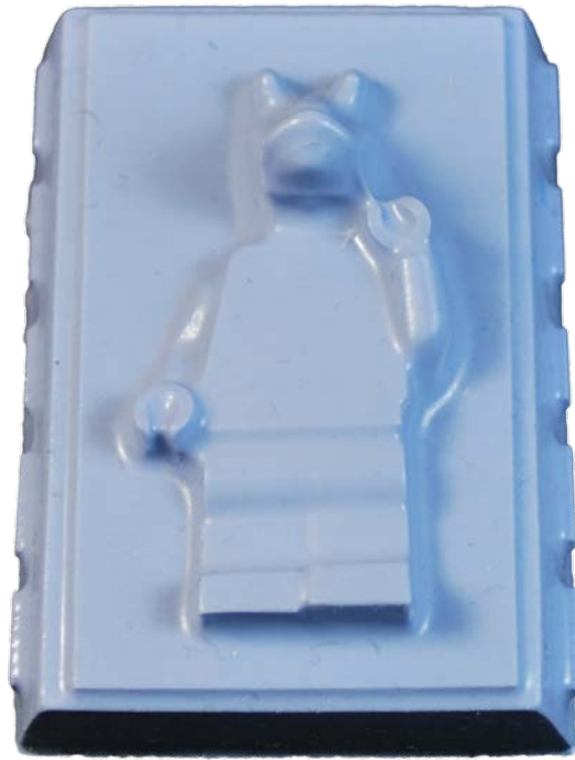
Rubber mold created from initial vacu-formed plaster Jar Jar.
