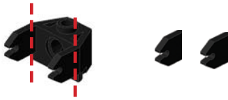
Cut or sand the body of the magnet holder off, leaving the arms to use.
