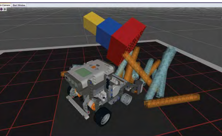
Robotsim is a real-time physics simulator, so things can fall and break, as this screen shows.
