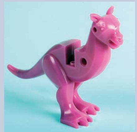
This pink Tuantuan body was produced to check for possible flaws in the mould that would lead to 'break points'. Most test moulding is done in red, but in this case a slightly transparent pink colour was used.
