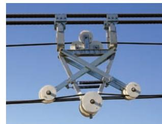
The cradle: the stabilizing arms retract upwards at carriage passage.
