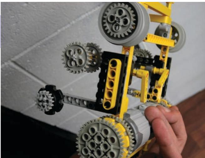
WALL•E's tread wheels. The motors (Power Functions XL) can be seen at the bottom of the photo.
