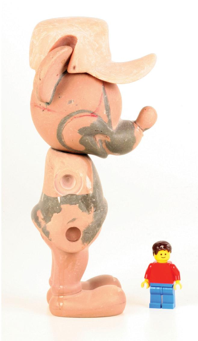
LEGO Designer Dan Villa Serber worked with the 3:1 scale models for the LEGO system Disney figures. During the development process of new figures, they are first sculpted by hand, then scanned and later printed in a 3D printer.
