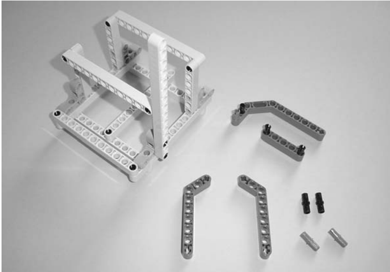
Figure 11-37. Connect the 15-hole beam to the cage to hold the motor.
