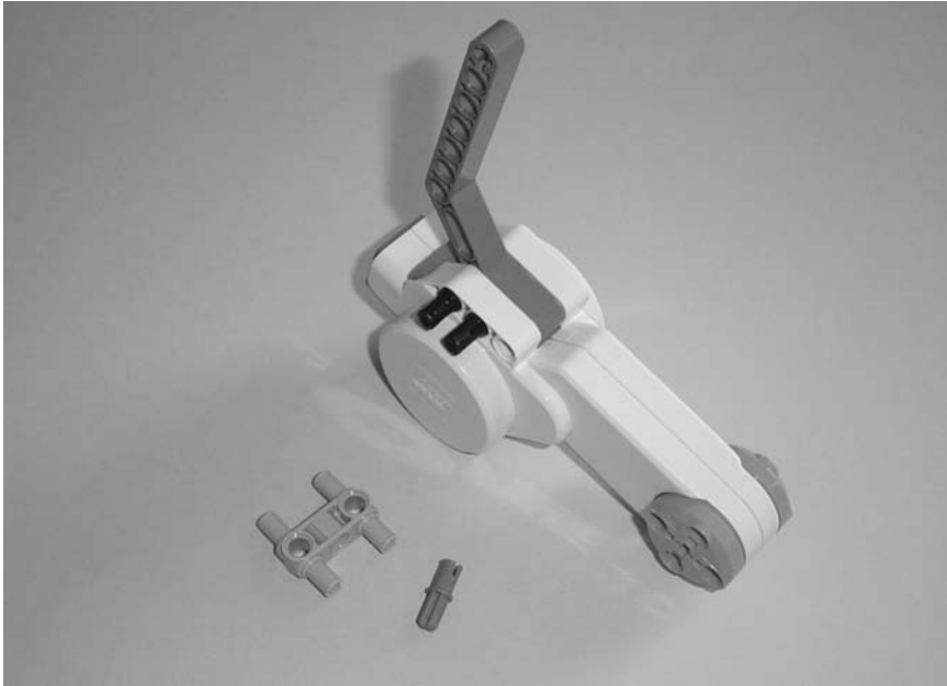
Figure 15-3. Place the long black connectors in the motor as shown to secure the angled gray component.
