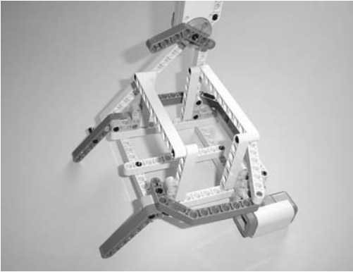
Figure 11-49. Connect the gray component to the motor as shown. This is the arm that will press on the camera button.
