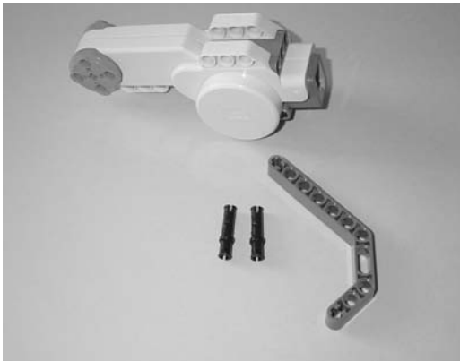
Figure 15-8. Starting components for the main body's other wheel assembly
