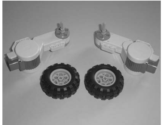
Figure 19-32. Insert the rods into the motors and secure them with the small bushings.
