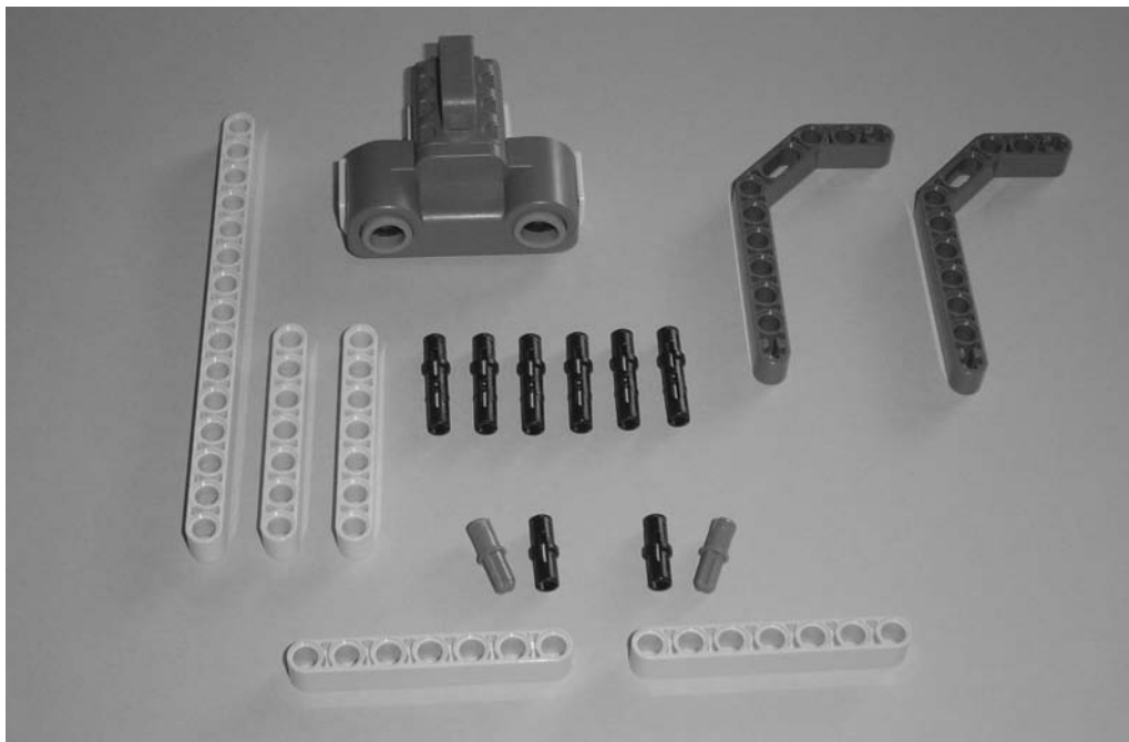
Figure 19-34. Use these components to build the neck/Ultrasonic Sensor assembly.
