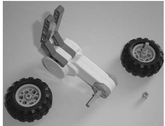
Figure 15-5. Insert the axle rod into the motor and slide the bushing on. Connect the other angled gray component as shown.
