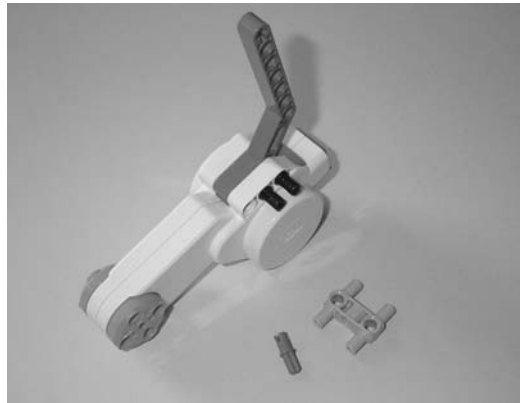
Figure 15-9. Place the long black connectors in the motor as shown to secure the angled gray component.
