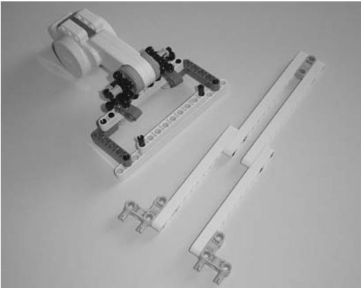
Figure 19-21. The vertical support bar will connect to the motor/cage-arm assembly.
