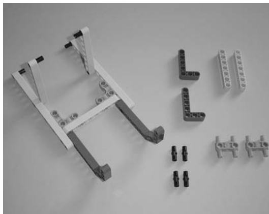
Figure 15-28. Connect the two 9-hole beams and the two angled gray beams to the main lifting mechanism as shown.
