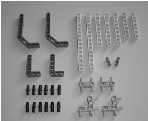
Figure 15-25. The components used to make the lifting arm mechanism
