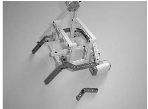
Figure 11-48. Place the blue connector and small black connector in the gray component.
