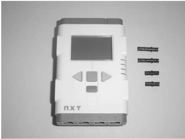
Figure 3-10. The body will be made of the Intelligent Brick and a few connectors.
