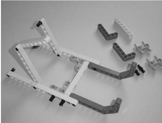
Figure 15-29. On one side, insert two small black connectors and connect one 7-hole beam as shown.
