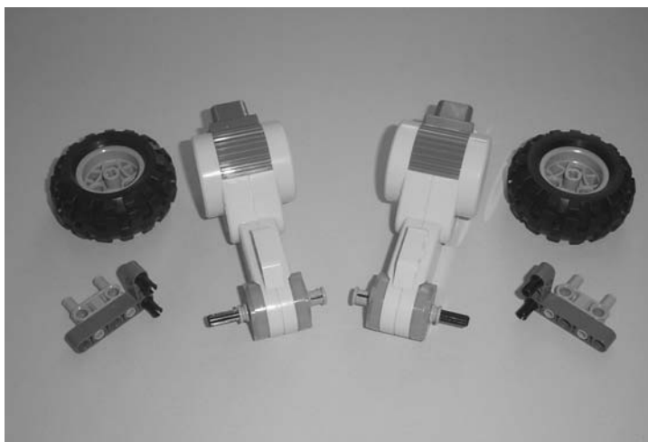
Figure 3-13. Partial assembly of the left and right motor/wheel combinations
