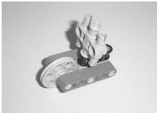
Figure 3-24. The final rear-wheel assembly—set this aside for now
