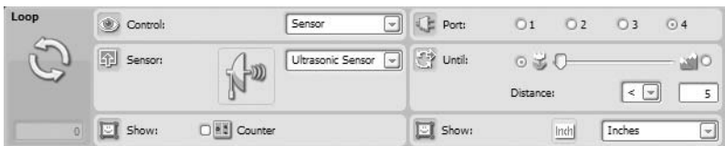
Figure 4-11. Use the configuration panel to configure the inner LOOP block.
