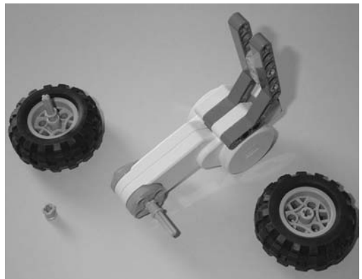
Figure 15-11. Insert the axle rod into the motor and slide the bushing on. Connect the other angled gray component as shown.
