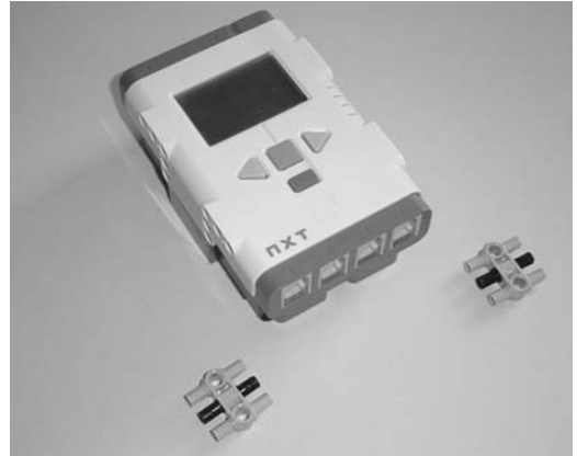
Figure 15-15. Insert the long black connectors into the gray pins.
