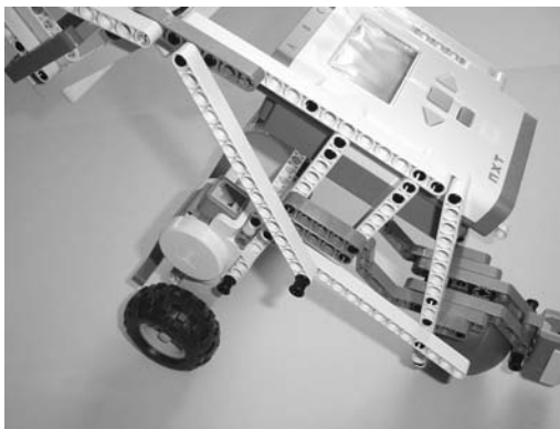
Figure 11-57. Connect the 15-hole beam to the main body.
