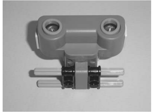
Figure 3-3. The fully assembled ExploroBot head—set this aside for now
