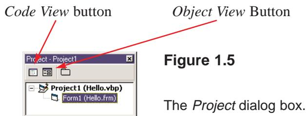
The two icons indicated above are useful for switching between the Object and Code views of the object.
