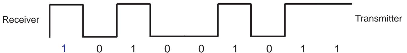
However, as you can see from the above diagram, the data sequence ends with a '1'. Because the start bit is also a '1', we want the intervening period between data transmissions to be at logic level '0'. In order to ensure that this happens, we include a 'stop bit' at the end of the data transmission, which is, of course, at logic level '0'. The data packet as it stands now is presented below.
