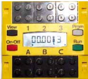
There are three motor outputs on the RCX. These are black connectors which are labelled A, B and C. You can connect the electrical lead to each output in four different orientations. You can also connect the other end of the lead to the motor in four different orientations. Whichever orientation you choose can influence whether the motors rotate in a clockwise or anti-clockwise direction.
