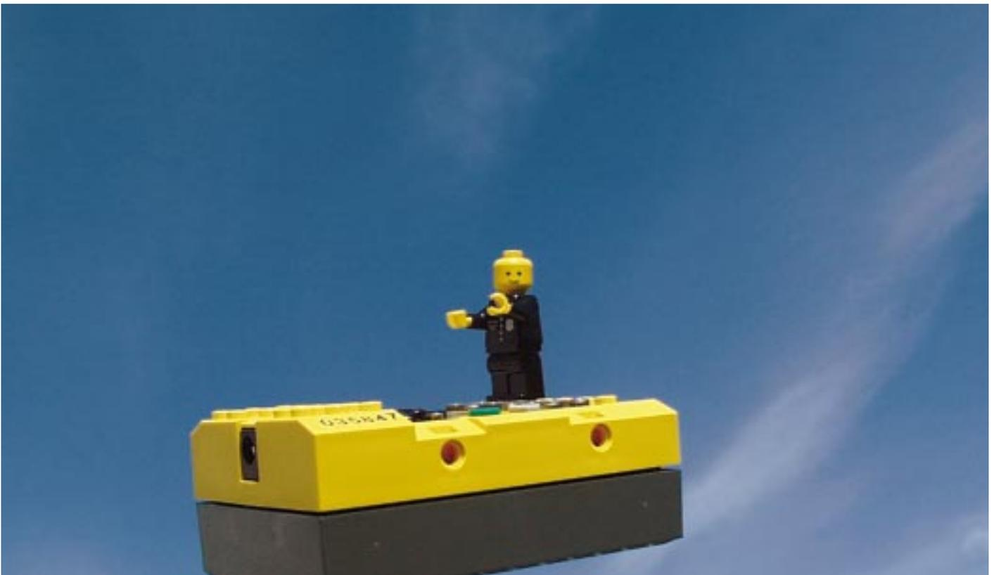
You will now be introduced to the Lego Mindstorms kit and how it is controlled by your programs. The kit comprises of several key elements which work together. The brain of the robots you will create is called the RCX, as shown.
