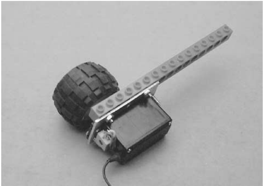
FIGURE 20.14 A servo mounted on a homemade servo bracket.
