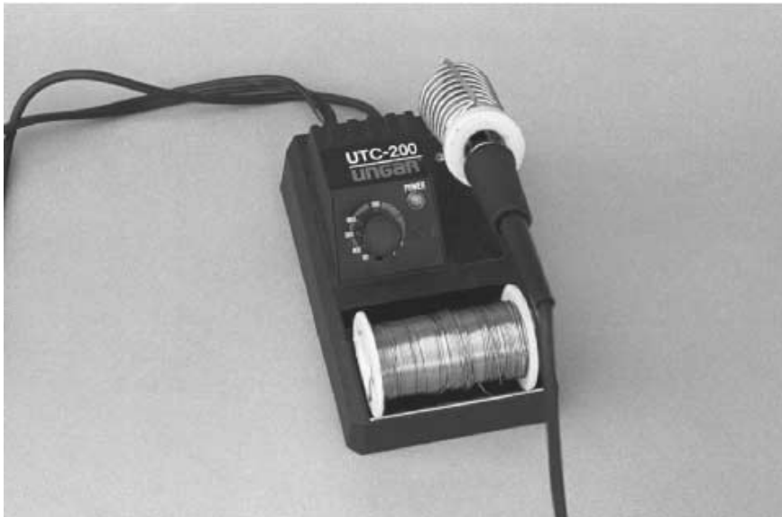
FIGURE 6.6 Use a low-wattage (25 to 30 watts) soldering pencil for all electronics work.
