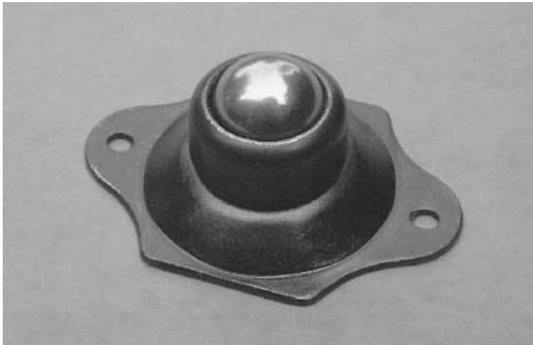
FIGURE 16.9 Ball casters (or ball transfers) are omnidirectional. For medium- to large-sized robots consider using them instead of wheeled casters.
