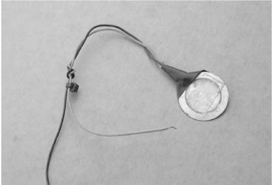
FIGURE 35.8 Piezo ceramic discs are ideally suited to be contact and pressure sensors for robotics.
