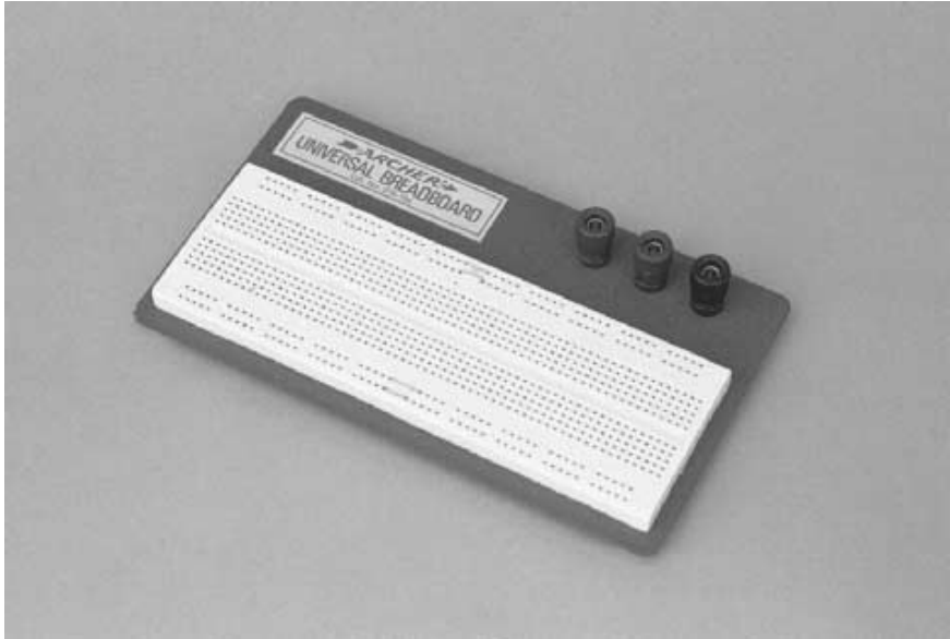
FIGURE 3.4 Solderless breadboards are used to “try out” a circuit before soldering. Some robot makers even use them in their final prototypes.
