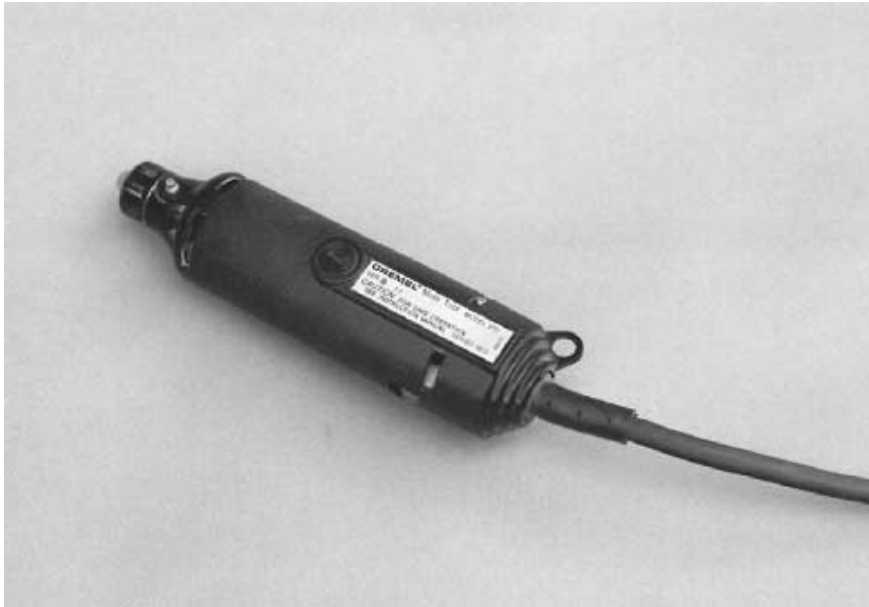
FIGURE 3.1 A motorized hobby tool is ideal for drilling, sanding, and shaping small parts.
