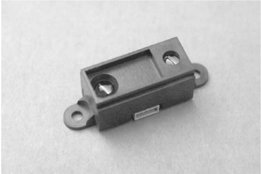
FIGURE 38.15 The Sharp infrared sensors are equipped with a focused infrared light source and a linear photodetector array. Distance can be determined by detecting where the reflected light touches the array.
