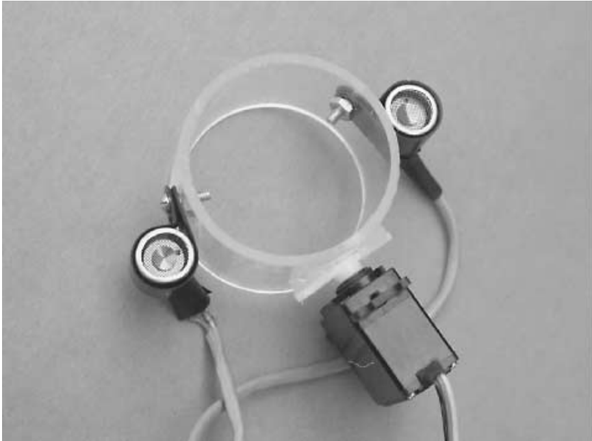
FIGURE 36.9 Ultrasonic sensors mounted on an RC servo scanner turret.
