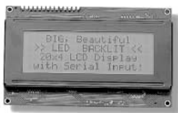
FIGURE 31.9 This LCD display connects to the Basic Stamp via a serial line and is programmed using simple PBasic statements.
