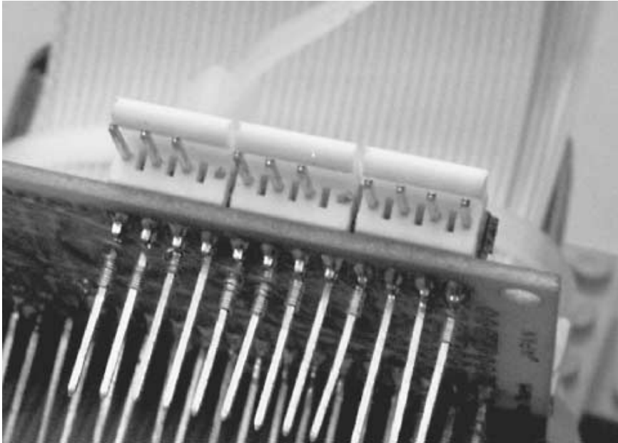
FIGURE 20.6 You can construct your own servo connectors using snap-off headers soldered to your robot control board.
