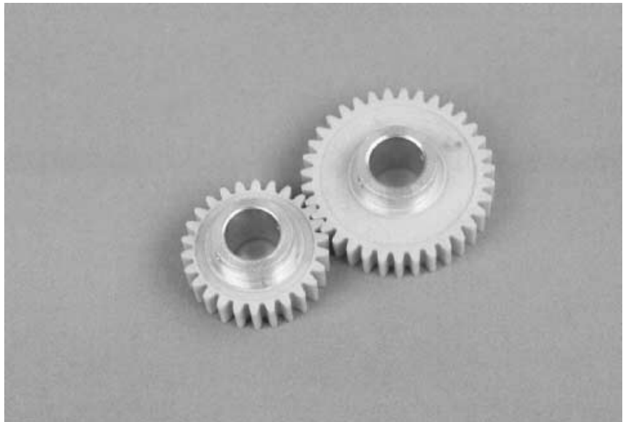
FIGURE 17.11 Spur gears. These particular gears are made of nylon and have aluminum hubs. It's better to use metal hubs in which the gear is secured to the shaft with a setscrew.
