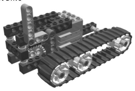
The left drive sub-assembly is almost a mirror image of the right drive sub-assembly, and includes the motor, gearbox, and tractor tread.
