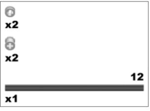
Pass a #12 axle through the beams and the liftarms. Secure it with two bushings on the outside.
