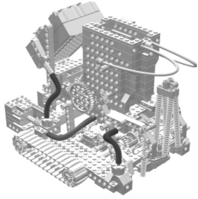
You will notice that there are some beam extensions and pegs with friction on either side of DominoBot. These pieces are the mounting points for the flexible hoses in this step. Hook up the TECHNIC flex hoses as shown here. Do the same on the opposite side, and you're done!
