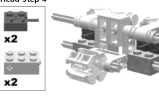
Connect a wire to each of the two touch sensors, and slide them onto the axle under the black liftarms. Once the bumpers are attached, the pivoting angle connectors will cause the bumper to push the touch sensor's yellow button when SumoBug encounters an obstacle.
