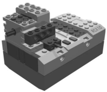
Connect the 2x4 plate to the RCX first to create a level platform for the motor. Next, connect the motor and the electrical wire to RCX Input Port 1. This wire will be attached to the touch sensor in a later step. Finish this step by attaching the 1x2 plate which will provide a level surface to attach the 1x4 TECHNIC brick.
