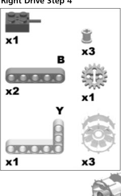
Slide the 16t gear onto the front axle. Mount the sprocket wheels on to the axles with a bushing on each to hold them in place.
