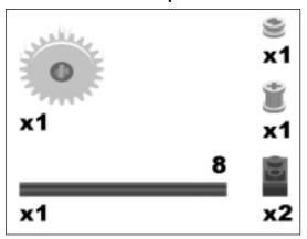
Slide the white clutch gear and the bushing onto the #8 axle, then attach it to the motor through the black 1x4 beam. A half-bushing holds the axle in place on the other side of the beam.
