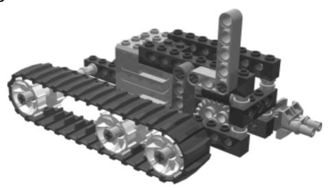
To begin, you will build the right drive sub-assembly, which includes the motor, gearbox, and right tractor tread. The gearbox uses a worm gear and a 24t gear to reduce the rotation speed by a ratio of 24:1. In other words, for every 24 revolutions of the motor, the wheel inside the tractor tread turns only once.
