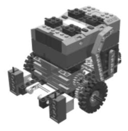
With two light sensors, line following is a cinch. Nessie will negotiate a sharp 90-degree bend in both a clockwise and counter-clockwise direction. Furthermore, Nessie can be programmed to detect a T-junction on the line, where she can be made to stop, change direction, or carry out a specified task such as dumping a cargo into a receptacle.
