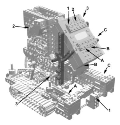
Insert the RCX. Using the diagram, match the numbers and letters. For example, RCX sensor Port 2 should go to the loader sensor Port 2 (at the top left). The light sensor has a short cable. In order for it to connect to sensor Port 1, use one of the provided medium length cables to extend its length. Connect RCX motor Port B to the loader main drive motor (below the RCX).
