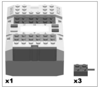
Attach the RCX to the top supporting plates of the robot base. To do so, separate the two sections of the RCX. Position the bottom section over the supporting plates and press down firmly. Replace the top section of the RCX (with the batteries) carefully over the bottom section.
