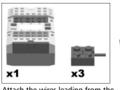
Attach the wires leading from the light sensor to Input Port 1. Attach the wires leading from the touch sensor to Input Port 3. Attach the wires leading from the motors to Output Port A and B.
