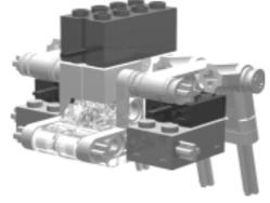
Slide the two touch sensors onto the axles, and attach the light sensor
