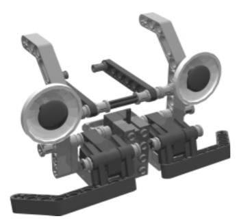
SumoBug's head is more than just a pretty face. It holds the light sensor and two bumpers equipped with touch sensors. During a match, SumoBug uses the light sensor to see the black line on the RIS Test Pad. Separate bumpers let SumoBug know which side the opponent is on.
