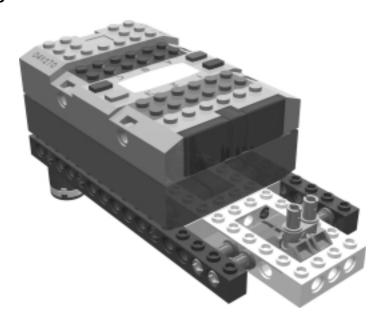
The chassis sub-assembly is the frame on which WideBot is built. It supports the RCX brick and provides a solid connection for the other parts. Using the open-centered transparent bricks, you can quickly build WideBot's sturdy frame.
