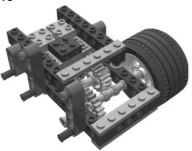
The left drive sub-assembly is a mirror image of the right drive sub-assembly, with the exception of the gearbox. To ensure that the wheels drive in the same direction, the gearbox setup is identical in both motor assemblies (that is, it is not a mirror of the right drive, but is exactly the same).
