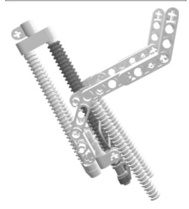
Insert the parts as shown, leaving the yellow elastic band for last. The elastic goes between the green and purple flex hoses and wraps around the black friction pegs (below) that are inserted in the yellow doublebent liftarm. Its purpose is to hold the purple hoses against the front of the loader mechanism. This is important, so study the image carefully.
