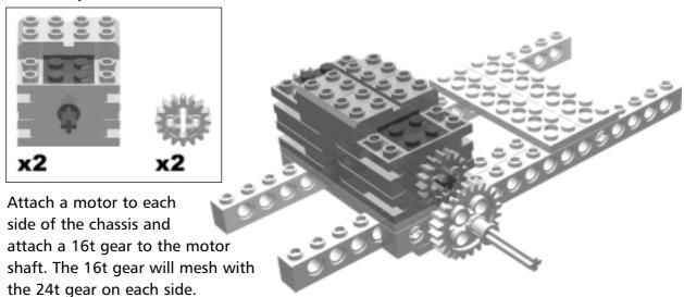
The meshing of the gears is not exact LEGO geometry; however, for practical purposes it is close enough.
