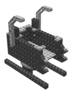
The bin holds items to be compacted. The sides contain the waste so that the ram can compress the waste.
