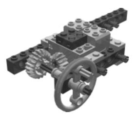
The right drive sub-assembly is a mirror image of the left drive sub-assembly.
