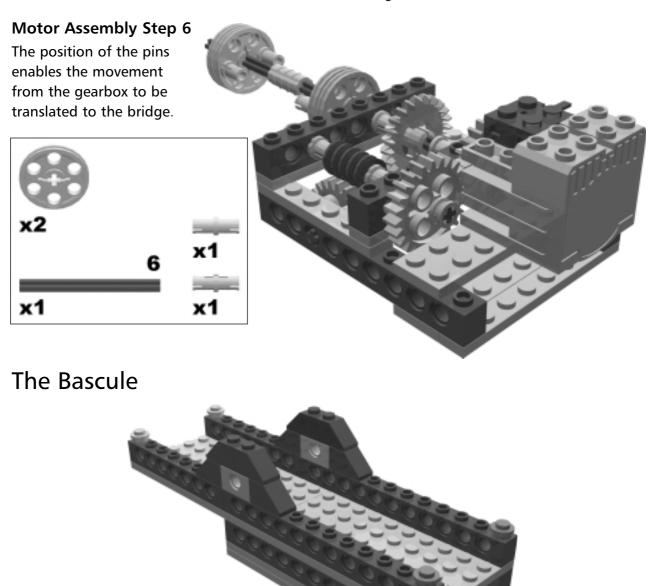
The Bascule sub-assembly is the moveable part of the bridge that will lift or draw. It is often also called a *balance*.
