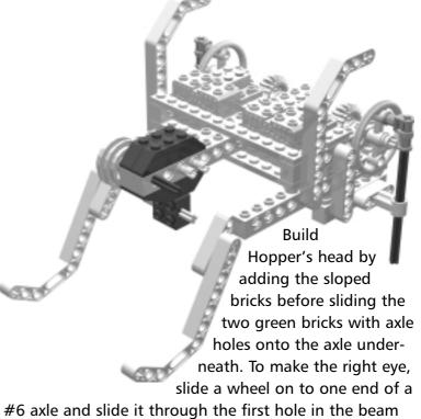
Using the #10 axles and bushings, build the legs on both sides of the robot.
