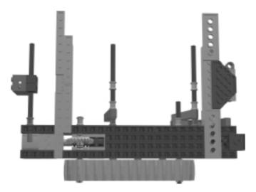
The left drive sub-assembly connects to the right drive sub-assembly to form the driving base of the DominoBot. Or course, its purpose is to give it mobility.
