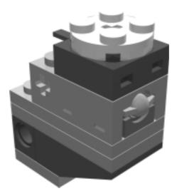
The loader sensor sub-assembly completes the essential function of identifying to the RCX when the loader mechanism has dispensed a domino, and when the loader has reset and is ready for the next domino.
