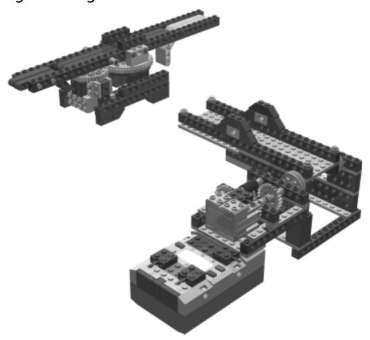
The final steps include addition of the RCX, and snapping together of all of the previously built sub-assemblies. The RCX controls the movement of the Drawbridge and Island Footbridge, and sounds warning tones to let others know when the Drawbridge is lifting, lowering, and when it is safe again for traffic to cross.
