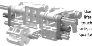
Use the 1x3 grey liftarms to secure the touch sensors on each side, and add the three-quarter-length pins.
