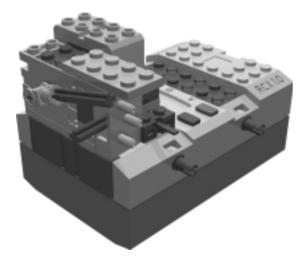
The RCX Air Compressor Control sub-assembly controls the flow of air. The RCX is programmed to power the motor when the touch sensor is pressed.
