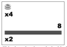
Slide the axles through the black axle joiners, then add the half-bushings. The axles provide the connection points for the grabber's motor sub-assembly, which you will build next.
