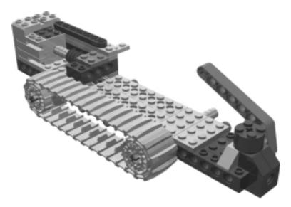
The right drive sub-assembly provides motion to the DominoBot. Tracks provide the ability to turn on a tight radius.
