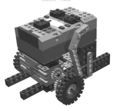
At first glance, Nellie closely resembles Robot 5, Nessie. However, as you build this robot you will see that Nellie employs a significant change in how it moves by replacing the caster wheel with a sliding rear wheel. Nessie used a freely movable caster to give it great maneuverability for turning, which is advantageous for line following. However, as you may have already realized, following a straight line offers results that could be considered poor.
