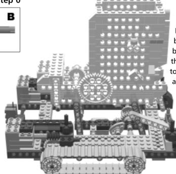
Locate the loader and base sub-assemblies built earlier. Connect the loader sub-assembly to the base sub-assembly using four, long, blue friction pegs. Take note of the location where the pegs are inserted. It is the same on both sides.
