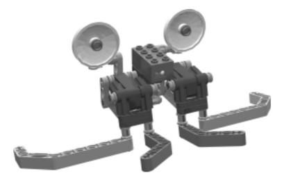
The head sub-assembly provides WideBot with two senses: touch and sensitivity to light. With touch sensors behind the left and right bumpers, WideBot can respond appropriately when it bumps into an object. The light sensor measures brightness directly ahead.
