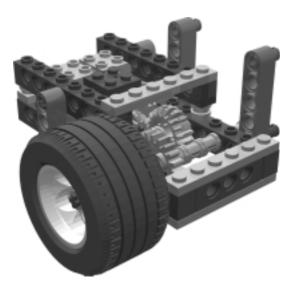
The right drive sub-assembly is a complete drive unit that includes the motor, gearbox, and right wheel. The gearbox turns the rotation angle 90 degrees and reduces the rotation speed by a ratio of 5:1. In other words, for every five revolutions of the motor, the wheel turns only once.
