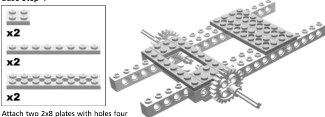
studs from the end of the rear TECHNIC beams as shown.
