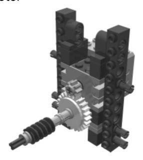
The grabber motor sub-assembly powers the grabber arms using a worm gear.
