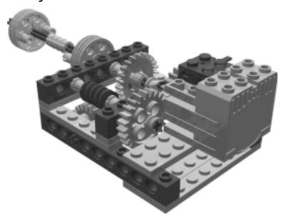
The motor assembly includes a gearbox with two worm gears that provide low speed and high torque, which is exactly what is needed to lift the heavy bascule.
