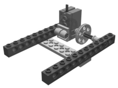
The sliding wheel and rotation sensor are incorporated in this sub-assembly, which is then attached to the main robot base.
