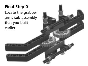
This step may be a little tricky. Locate the grabber motor sub-assembly that you built earlier, and slip the motor's axle with the worm gear between the two 24t gears. The axle should fit securely inside the blue axle connector on the front of the grabbers. The worm screw should mesh with the gray gears.
