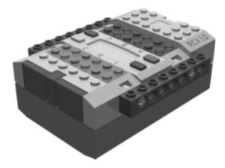
The RCX brick needs a beam on either side so that it can be attached to the body of the robot.
