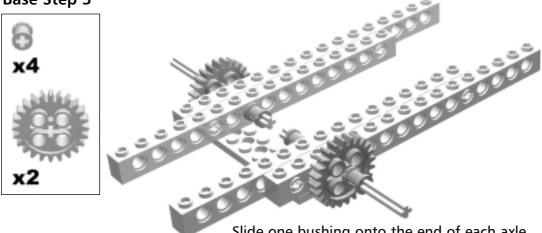
Slide one bushing onto the end of each axle located in the interior of the base frame.
