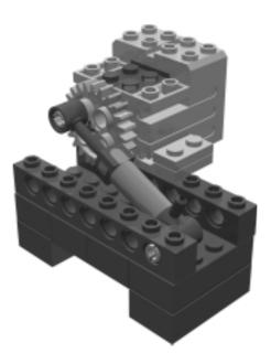
The compressor sub-assembly consists of a motor with a gear. This will move the pump in and out to create air pressure; the air will then be pushed through the tubing to move the piston.
