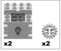
The motor has been raised one plate high to allow the 16t gear to mesh with the 24t gear.
