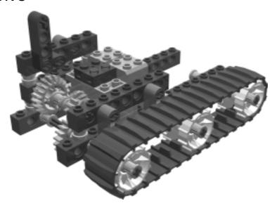
The left drive sub-assembly mirrors the right drive sub-assembly, but notice that the gears are exactly the same in both modules. This ensures that the wheels drive in the same direction when the motors run forward.
