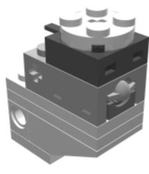
The white circular plate has an important function. In **Final Step 6**, you will insert a yellow flex tube from the loader to this plate. This will provide spring to the sensor unit to allow it to consistently maintain accurate readings while dominoes are being dispensed.
