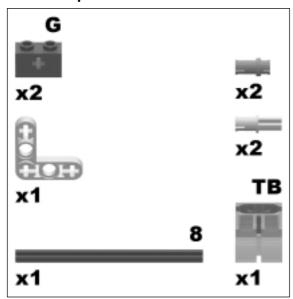
Assemble the parts on the transparent blue connector block. The green bricks with axle holes are the attachment point for the light sensor.
