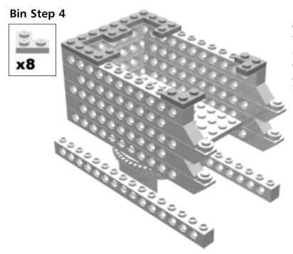
Add the corner pieces to guide the ram as it moves up and down. These corner pieces work with the 2x2 bricks that you have the option of adding in **Pneumatic Ram Step 0**.
