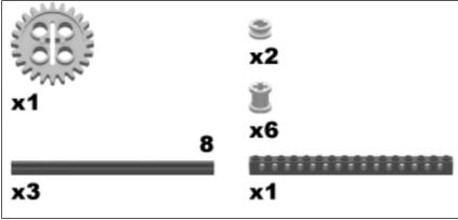
Slide the axles through the holes in the 1x16 TECHNIC brick. Add the bushings and the 24t gear to hold the axles in place. The 24t gear is secured on the axle with the half-bushings.
