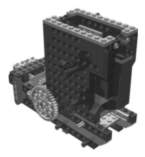
The loader sub-assembly delivers a domino from the stack to the loader arm by using a push mechanism. It also uses a touch sensor to alert the program that a domino has been delivered.
