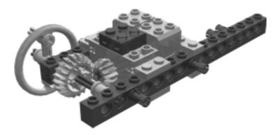
The left drive and right drive sub-assemblies are used to rotate the large pulley wheels which provide the hopping action for the legs. The beveled gears turn the angle of rotation 90 degrees and reduce the speed.
