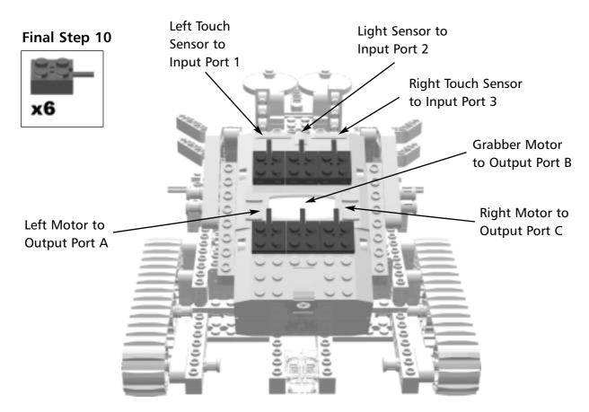
Connect the wires to the RCX brick as shown.
