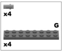
Place four 2x8 green plates to form the support for the RCX. Insert a pair of dark gray three-quarter length pins to each side of the vertically stacked 1x4 beams.
