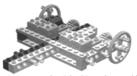
Locate the right drive sub-assembly and attach it to the left drive subassembly as shown.
