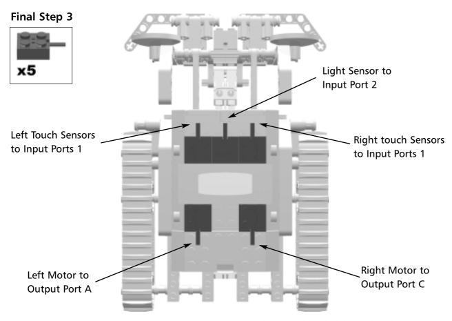
Now it's time to connect the wires to the RCX brick. Connect the left and right touch sensors to Input Ports 1 and 3, and connect the light sensor to Input Port 2. Connect the left motor to Output Port A and the right motor to Output Port C, making sure that the wires are oriented as shown.
