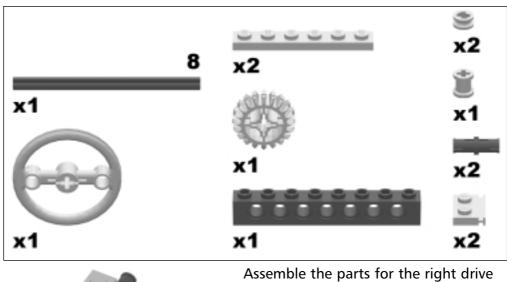
sub-assembly as you did for the left drive sub-assembly. Notice that the arrangement of gears is identical to that of the left drive sub-assembly. This ensures that the motors turn in the same direction.
