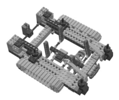
The base sub-assembly consists of the left drive sub-assembly, the right Drive sub-assembly, and the distance sensor sub-assembly. You will connect them together in the following series of steps.
