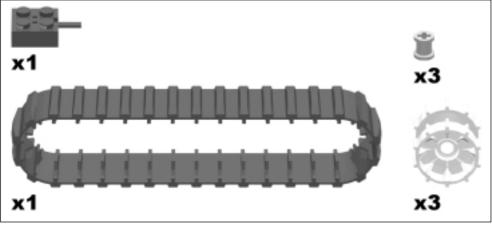
Add the sprocket wheels and the tractor tread as shown. Secure sprocket wheels with bushings. When you connect the wire to the motor, make sure that the wire points toward the back of the motor.
