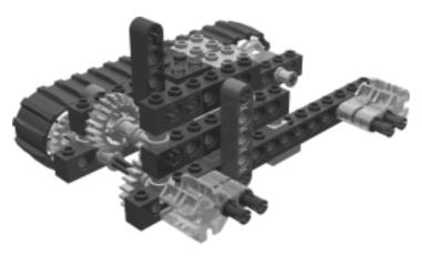
The right drive sub-assembly includes the motor, gearbox, and right tractor tread. The gearbox reduces the rotation speed to a one-fifth of the motor's speed.
