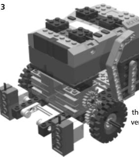
Attach a light sensor to the bottom of each of the blue 2x2 plates. Attach the wires from the light sensors to Output Ports 1 and 3. The direction of the wires at the Input Ports is immaterial.
