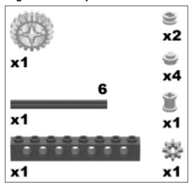
Slide a #6 axle through the first hole of the 1x8 TECHNIC brick and secure the axle with a half-bushing.
