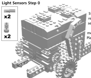
Start with the main robot base with rear sliding wheel and rotation sensor.
