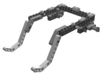
Hopper is a four-legged robot designed to move in a loping, hopping motion. Unlike most robots with legs, Hopper's design is extremely simple, which makes it an excellent starter project, and its unique gait makes it a fun robot to play with and program.
