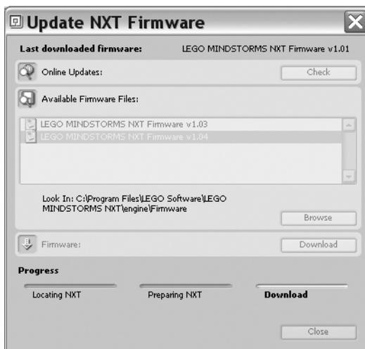
Figure A-3. Updating the NXT firmware on the Brick
