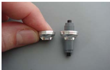
Figure 9. Making a holding fixture for the reflector.
