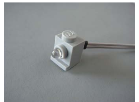
Figure 5. Fitting a LifeLite in a headlight brick.
