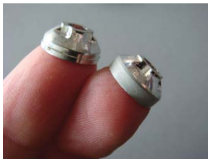
Figure 11. Ground reflector (right) compared to the original.
