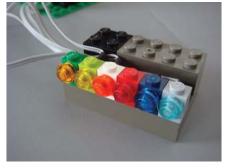
Figure 2. Lifelites installed inside headlight bricks.
