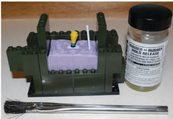
Figure 5. Disassemble the mold box for Klean Klay clean up. Reassemble the mold box. Coat the top with rubber to rubber mold release and pour the second half of the mold.
