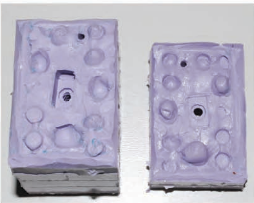
Figure 6. The finished mold with original and replica cast parts.
