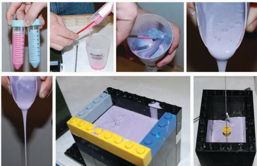
Figure 4. Pour technique using the "V" shape and slow pour rate to remove air whipped into the silicon resulting from mixing the two parts together.
