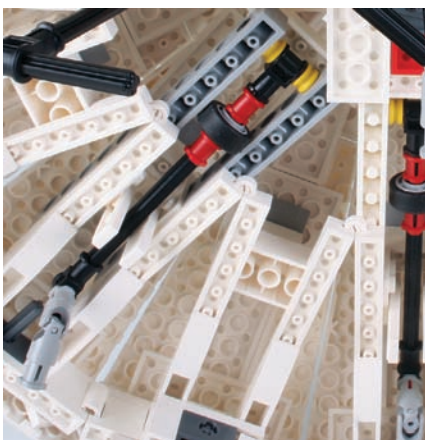
An early version of the mechanism that made the horses go up and down. The small wheel would roll over curves on top of the center pier.
