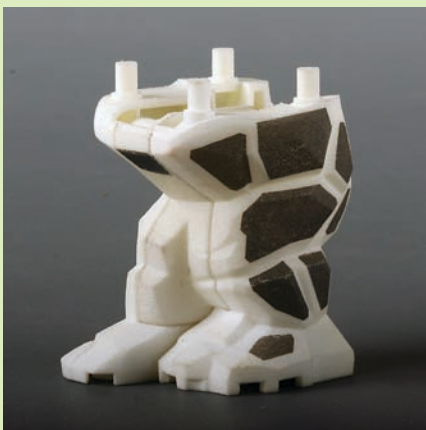
Midi-monster legs! The Mid-sized rock monster is made of several different moulds then joined together. This version was made to show where the legs needed to be printed.
