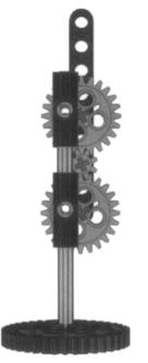
By driving any of the three gears, this simple leg will go up and down, forward and back, always in a circle. The leg always remains vertical. Figure 15.13 shows a slightly different approach, where only one point of the leg is attached to a wheel, and the leg itself slides freely into a rotating support (fulcrum).
