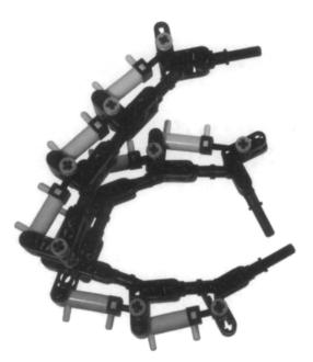
Figure 11.11 The Three-Finger Pneumatic Hand with Complete Tubing
