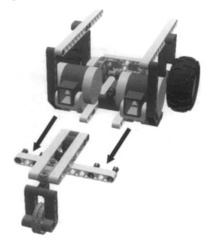
Figure 6.15 Separating the Left and Right Drive Assemblies
