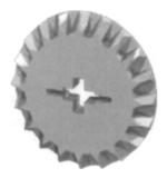
The 24t gear also exists in the form of a *crown gear*, a special gear with front teeth that can be used like an ordinary 24t, but can also combine with another straight gear to transmit motion in an orthogonal direction (that is, composed of right angles), possibly achieving at the same time a ratio different from 1:1 (Figure 2.12).
