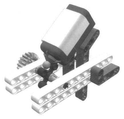
Making a rotation sensor out of a light sensor is not very different: Build some kind of rotating disk with sectors of different colors, and count the transitions from one color to the other (Figure 4.14). The general tip applies to this case too: Try to insulate the sensor from external light sources as much as possible.
