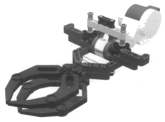
What if you need a compact, lightweight grabber? The flex system we briefly described in Chapter 9 allows you to transfer motion to distant parts, away from the motors and gears. Figure 11.7 shows a small operating hand based on this technique. A pair of opposing rubber bands introduces a degree of elasticity into the system, and helps the fingers return to their default setting once the hand comes to rest in its open position.
