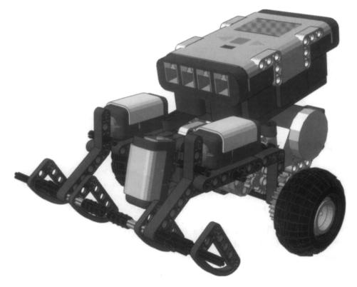
You can easily swap the ultrasonic sensor for a light sensor, which is attached to the structure with a long pin. Observing the result, the light sensor is now fairly far from the floor. The distance of the sensor from the pad is very important. Therefore, you should lower the attach point for the light sensor so that the sensor is much closer. Our experience teaches us that for the best results, this distance should fall in the range of 5 mm to 10 mm.
