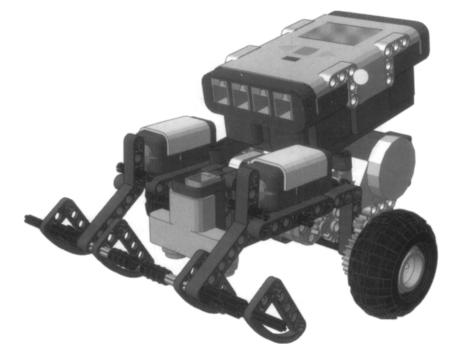
Unfortunately, this system doesn't cover all possible scenarios, because your robot could approach the edge at an angle that allows a wheel over the edge before detection occurs. You can improve upon the design and avoid this by providing the robot with two left- and rightedge sensors, but you'll probably have to give up the double bumper and go with a single sensor bumper.
