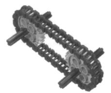
TECHNIC tread links can be used to make tracked robots (see Figure 2.24). However, like most LEGO parts, they are plastic. They provide very little grip when on slippery surfaces such as wood, tile, or plastic. They work better on other surfaces such as carpet.
