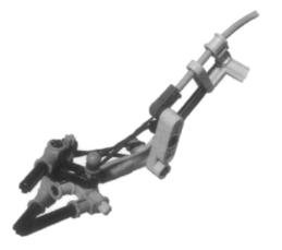
Try to use short fingers whenever possible. An object held by long fingers exerts more torque on the gears, just as a long lever makes lifting a heavy weight easier.
