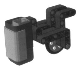
The front fork is driven by a steering assembly based on a worm gear, a 24t and two pulleys. As you learned in Chapter 2, the pulley-belt systems prevent any stall situation if the robot doesn't control the steering wheel properly when the software is not yet fully tested and debugged (Figure 14.11).
