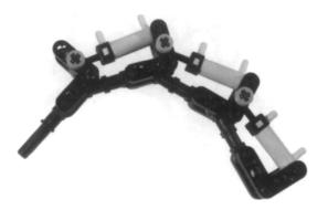
Figure 11.10 A Three-Finger Pneumatic Hand
