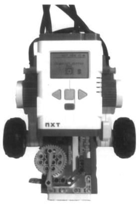
Of course, you might ask why you should bother creating a crude analog measurement device such as this when you can use the NXT display to simply show the rotation values for each motor. Good idea! Figure 9.6 is a sample NXT-G program that will drive the aforementioned robot forward for a period of time and display the encoder values for both motors on the screen.
