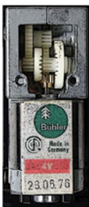
The Bühler 4.5V motor drives the left (smaller) gearwheel. Alternatively the 12V motor drives the right (larger) gearwheel. Due to the design of the gear the 12V engine runs much faster. The idea is now to replace an old 4.5V motor by a new strong 12V motor but to use the lower (4.5V) transmission ratio to make it useful to run with large spoke wheels!
