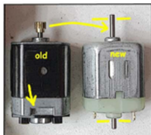
Two make the new motor fit, we need to (1) mill the gap at the bottom that holds the motor on the gear (see left) (2) cut the axles (3) transfer the brass gearwheel and (4) fix the electric contacts.
