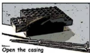
Open the casing by unscrewing the two upper screws
