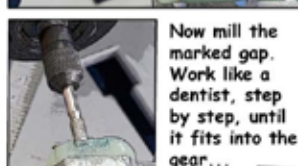
Next mark the gap to be milled at the printed side (engraving SUN) for correct polarity lateron
