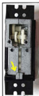
Two make the new motor fit, we need to (1) mill the gap at the bottom that holds the motor on the gear (see left) (2) cut the axles (3) transfer the brass gearwheel and (4) fix the electric contacts.
