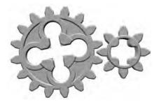
Figure 9-17: In this example, assume that the gear on the left is the driver and the one on the right is the driven gear. This demonstrates a high gear ratio that is fast but less powerful.
