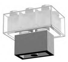
Figure 1-22: Studs inserted into tubes, not alongside them
