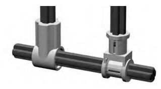
Figure 9-11: Rotating versus nonrotating openings in Technic couplers. The part on the left allows the axle to spin if needed, while the piece on the right keeps it from doing any spinning at all.
