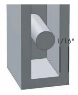
Figure 5-13: Standard LEGO bricks have walls that are approximately 1/16 of an inch thick.
