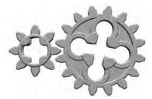
Figure 9-16: In this example, assume that the gear on the left is the driver and the one on the right is the driven gear. This demonstrates a low gear ratio that is slow but powerful.
